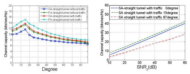
Fig 1. The average capacities of MIMO-SA and MIMO-PA system Fig 2. The average capacities of MIMO-SA system
